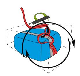
If the emergency parachute does not have a snug fit inside the rescue pocket, it could potentially rotate on itself while using the harness. The risers then roll up around the rescue parachute pod handle and prevent a deployment.
